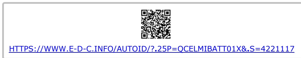
Fig. 8 Demonstration example of an AutoID URL encoded in ISO/IEC 18004 QR for opening the related WEB page by URL root, product number and serial number.
