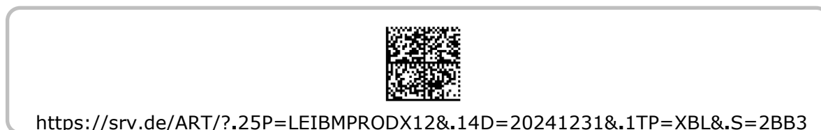
Fig. 3 Data Matrix Code carrying the AutoID URL of Table 5.
