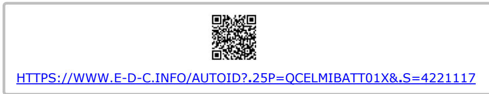
Fig. 7 Demonstration example of an AutoID URL encoded in ISO/IEC 18004 QR for opening the related WEB page by URL root, product number and serial number.
