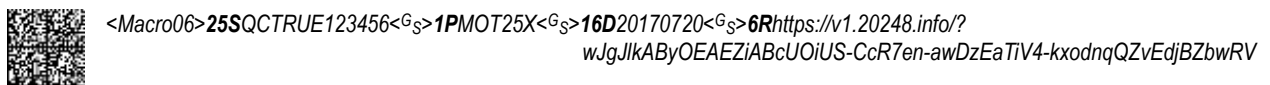
Fig. 41) ISO/IEC 16022 Data Matrix with object data and DigSig, size 40x40 Module, with X 0,25 = 10x10mm
