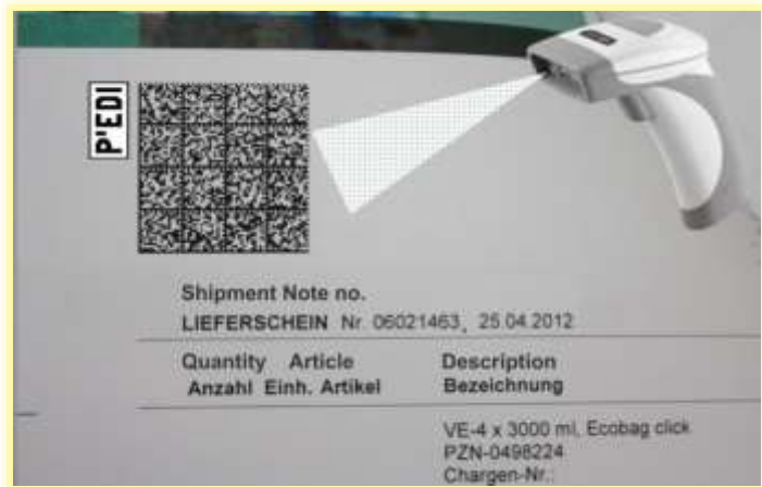
Fig. 30b) Shipment note applied with Data Matrix as P’EDI code carrying all product data of the shipment →
