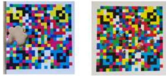
Fig. 11) JAB Code with LDPC check good for blobs and crumbs, source: SC31/JTC1/SC 31/WG1
