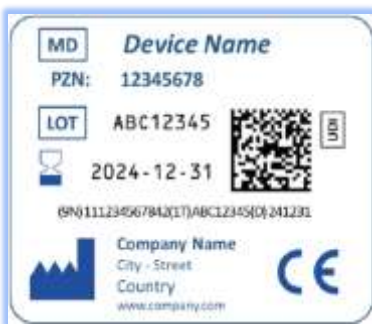
Fig. 31) MD label applied with UDI in IFA Coding System structure, source https://www.ifaffm.de/en/ifa-codingsystem/udi/udi_issuing_entity.html
