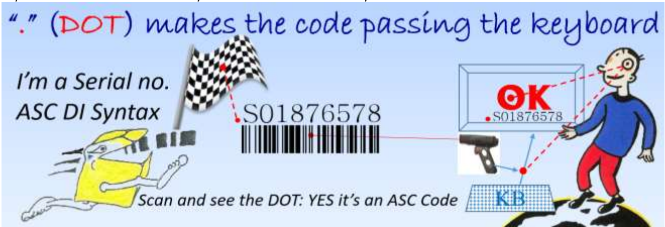
Fig. 39) The solution: The Flag Character "." (dot) makes the barcode data unique and passing keyboard & web interfaces
