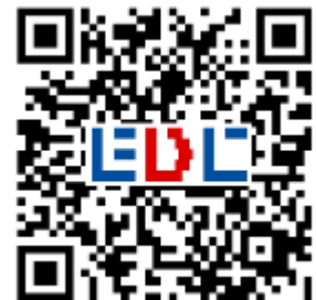
Fig. 32) Logo optically visible on the code and digital logo in the code “.5RQCDA:.....” →
