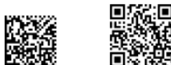
Fig. 31) Example → 5RQC... encoded with Data Matrix and/or QR Code (with same dot size)
