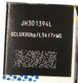
Fig. 33b) AIM DotCode placed on unit level package source: Incert
