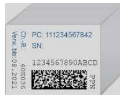
Fig. 28) Pharma Product Number (PPN) encoded in DIN 16587 DMRE
