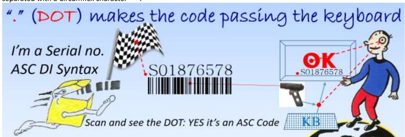
Fig. 26) Solution: The Flag Character "." (Dot) makes the barcode data unique and passing keyboard & web interfaces
