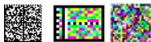
Fig. 14) From black and white to color: Data Matrix, Ultracode and JAB-Code (Click the symbols for more information)
