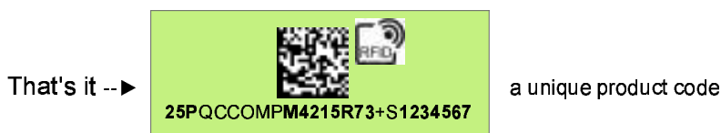
Fig. 23) Uniquely serialized product code in Data Matrix and RFID
