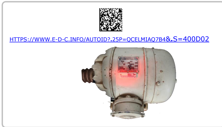
Fig. 9 Demonstration example of an AutoID URL encoded in ISO/IEC16922 Data Matrix for opening the related WEB page displaying the data of a motor and prepared information.
