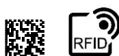
Fig. 3) Sample of a Data Matrix and emblem for an embedded RFID tag.
