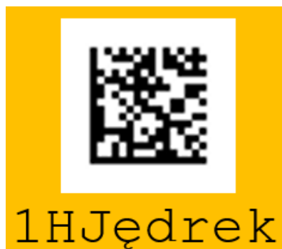
Fig. 8) Example DataMatrix with coded Polish name with ISO8859-2 character "ę".
